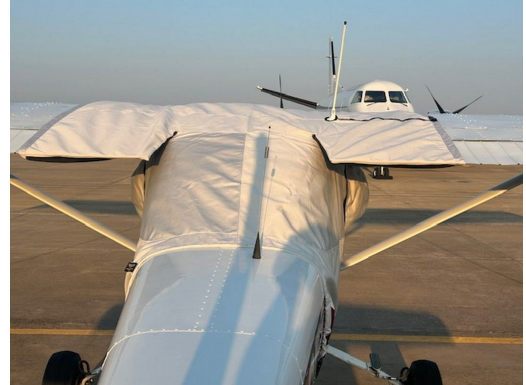
Cessna 150F Canopy Cover, over top type, extends to cover gas caps
