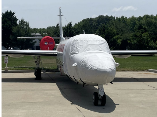
IAI 1124 Cockpit/Nose Cover Extended Aft Over Entry Door
