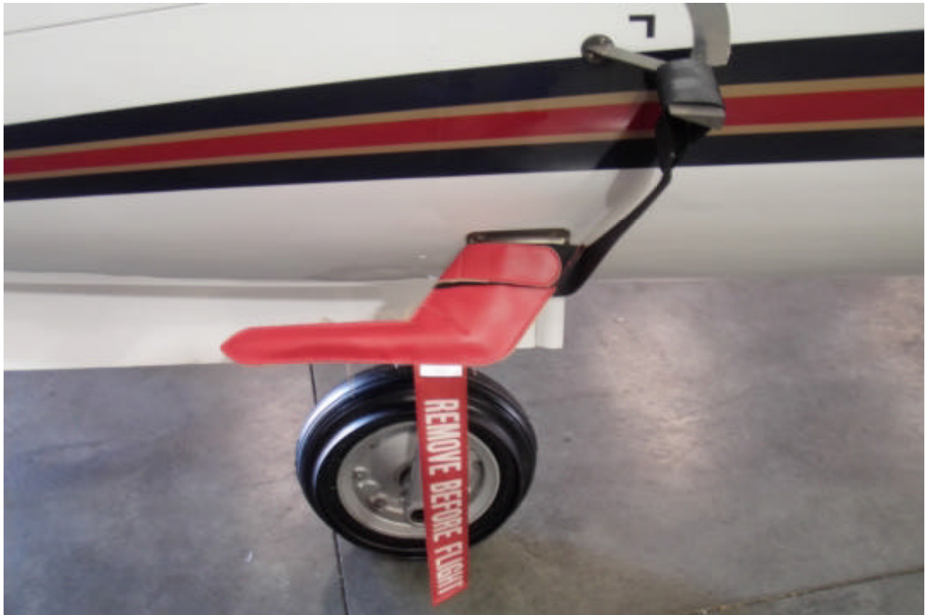
Learjet Non-burning Pitot Cover and AOA strap
