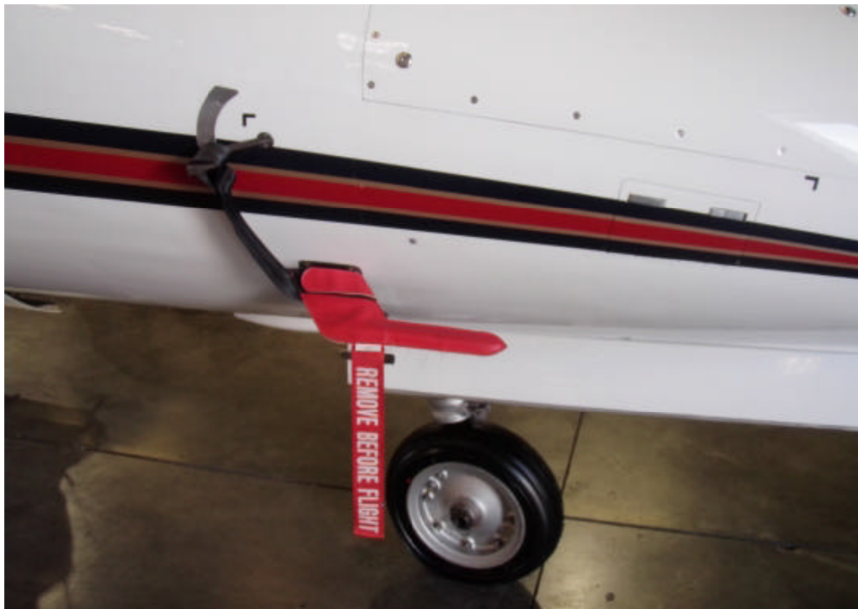
Learjet Non-burning Pitot Cover and AOA strap
