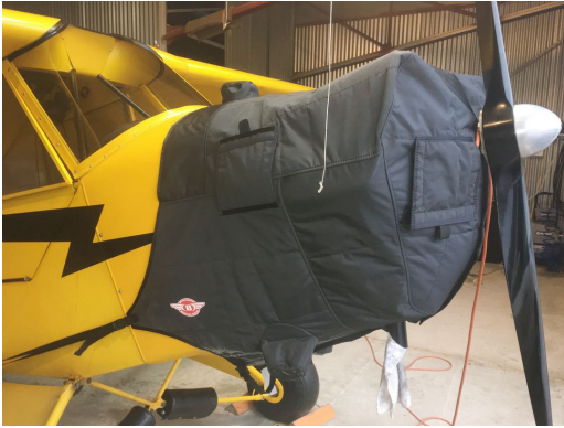
Piper J3 Cub Insulated Engine Cover
