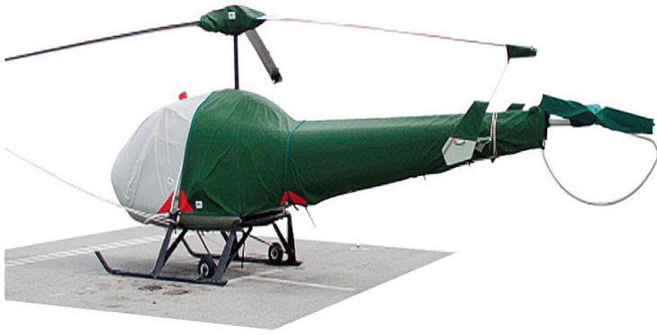
Enstrom 280FX Bubble, Engine, Tailboom, Main & Tail Rotor Covers Enstrom 280C Shark Bubble, Engine & Rotor Hub Covers
