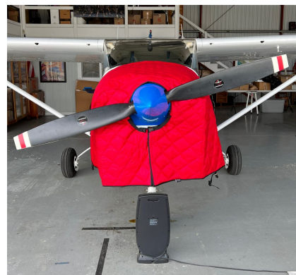
Insulated Hangar Blanket on Cessna 182
