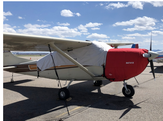
Cessna 206 Insulated Engine Cover, Canopy Cover
