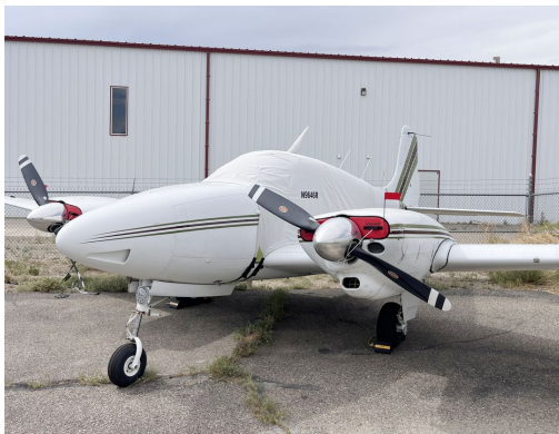
Beech B95 Extended Canopy Cover, Engine Plugs
