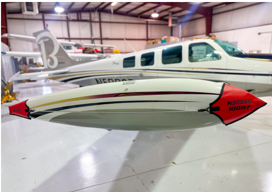
Beech A36 Fresh Air Inlet/Exhaust Plugs Tip Tank Safety Pads Beech A36 Fresh Air Inlet/Exhaust Plugs Tip Tank Safety Pads
