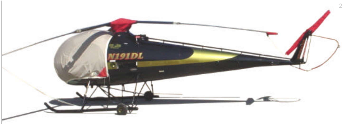
Brantly B2 Bubble, Main & Tail Rotor Covers & Tie-Downs
