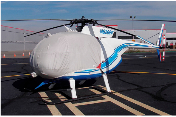
MD500C Bubble Cover with Wire Strike detail
