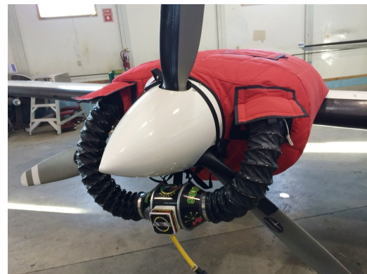
Cessna 402 Insulated Engine Cover with Heater
