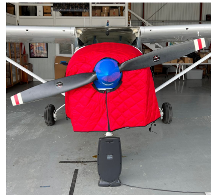
Insulated Hangar Blanket on Cessna 182
