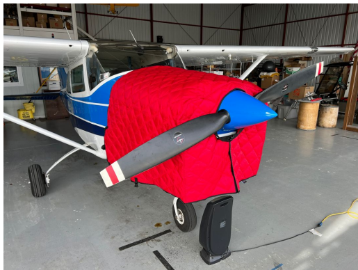
Insulated Hangar Blanket on Cessna 182
