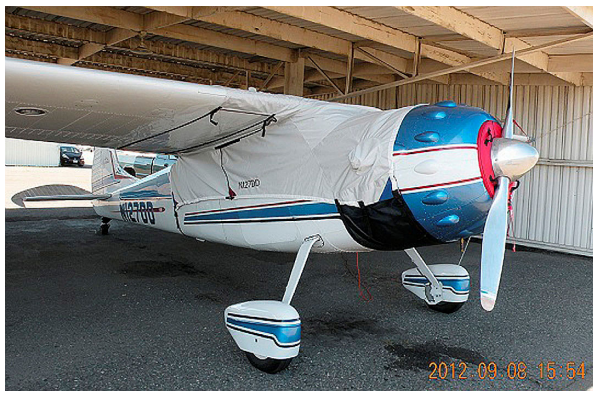
Cessna 195 Over-top Canopy Cover, 24" fwd ext to cover cowl ring gap, gas cap ext. & under belly cowl ring gap mesh covering
